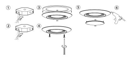
STEP 1 Prior to installation. Please install two screws (furnished) into the junction box. Do not drive screws completely to the end of the junction box.
