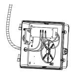
9.The top terminal connect the wire tube through the side hole to the L,N and G wires on the power supply.
