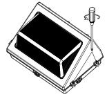
2.Use a screwdriver to remove the screws on both sides.
