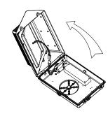
3. Open the fixture, disconnect the connection terminals, and remove the upper cover of the fixture.
