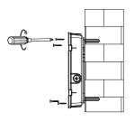
8.Push the expansion rubber plug into the mounting hole on the wall
