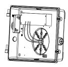
7. Thread the wire through the bottom hole.
