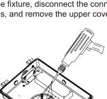
5. Drill through the mounting hole with an electric drill.
