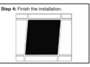
T-bar clips should be bent out to provide additional safety and support. Additional support may be required by local or national codes.
