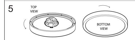
Using sticker on the fixture (reference point for mounting tab) and on the ceiling as reference point, lift fixture up to the ceiling and rotate clockwise until fixture is secured (45° turn until it locks).
