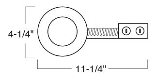
Cut-out: 4-3/8" ID: 4" Housing Length: 11-1/4" Housing Width: 4-1/4" Housing Height: 5-5/8"
