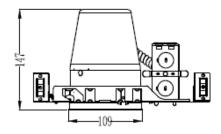
Minimum distance between edge of fixture and top of housing or other obstruction.
