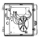
9.L,N and G wires connected to the power supply.
