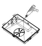
4.Drill through the mounting hole with an electric drill.
