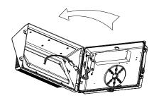
Open the fixture, disconnect the connection terminals, and remove the upper cover of the fixture.
