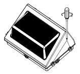
11. Fix the fixture with screws.
