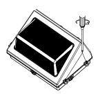
11. Fix the fixture with screws.
