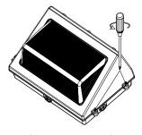
Use a screwdriver to remove the screws on both sides.
