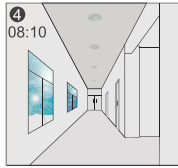
4 08:10 When the natural light level exceeds set point off to light, the light will turn off even when the space is occupied.
