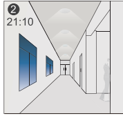
2 21:10 The light dims to stand-by level after the hold-time.
