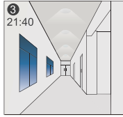
3 21:40 The light remains in dimming level at night.
