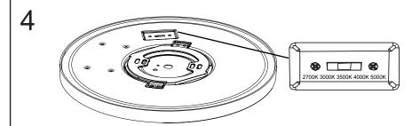
Attach provided to indents (opening) of the mounting tabs on back of the fixture with indents in the mounting bracket.
