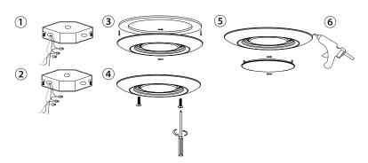
STEP 1 Prior to installation. Please install two screws (furnished) into the junction box. Do not drive screws completely to the end of the junction box. STEP 2 Connect supply wires to wires in fixture wiring box with proper size
