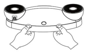
2. Knockout in back of mounting plate and push wires through the hole.
