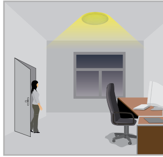
With insufficient natural light, the sensor switches on the light automatically when person enters the (options) standby level after the room. The lamp never switch off with presence, even the nature light is sufficient.
