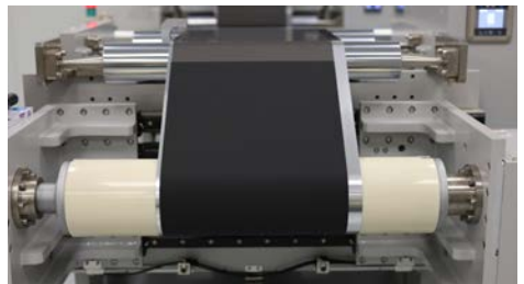
LFP cathode production at ONE Circle, Van Buren, MI.
