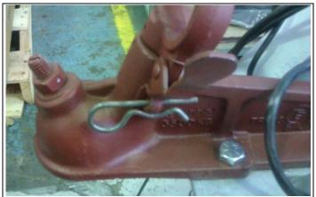
The "R" shaped safety pin was not fitted during this event but should have.
