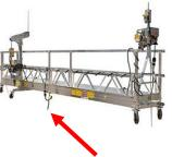
As part of the daily setup and throughout works, Swing Stage, operators are required to check that no cables can be entangled when the Swing Stage is in operation. Failure to visually check that the cable was clear when moving the cradle contributed to this incident. Cords should be supported in such a way to prevent the cradle from fouling or causing mechanical damage. All Swing Stage components should also be inspected for damage, wear and cracks, before use.
