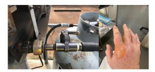
This incident is similar in nature to a previous incident where an employee received a cold burn when gas escaped from the hose while they were attempting to disconnect it from the bottle. Finding regarding this incident were also that suitable gloves were not worn and that first aid measures to treat the injury were not known.
