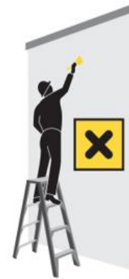
Never straddle or stand above the second tread below the top plate.
