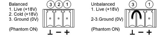
Microphones must be low impedance (200 to  $600\Omega$ ) and monophonic.
