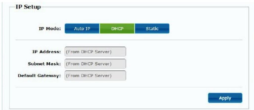
The screenshot shows the 'IP Setup' configuration page. At the top, there are three buttons for 'IP Mode': 'Auto IP', 'DHCP', and 'Static'. The 'DHCP' button is highlighted in green, indicating it is the selected mode. Below this, there are three input fields: 'IP Address', 'Subnet Mask', and 'Default Gateway'. Each of these fields contains the text '(From DHCP Server)'. At the bottom right of the form, there is a blue 'Apply' button.
