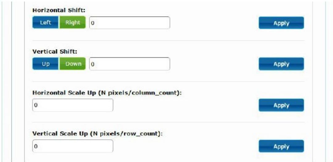
The screenshot shows a control panel with four sections for video adjustment:
