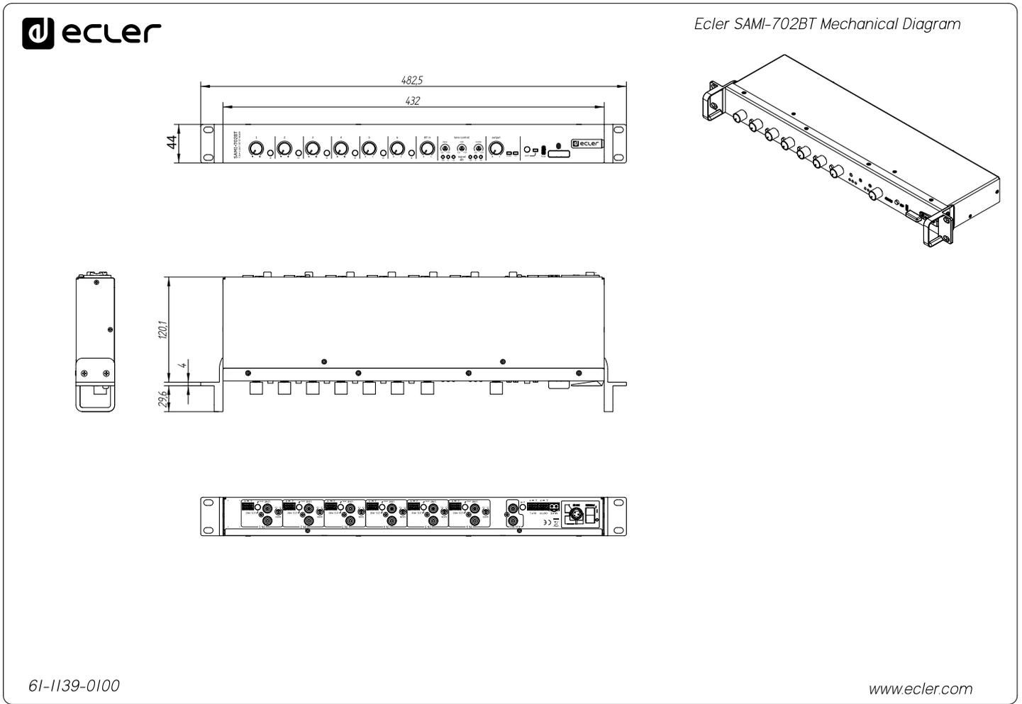
All the measurements are in mm
