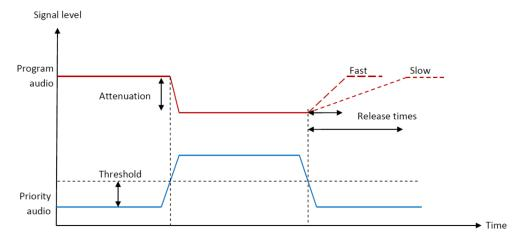
The priority mode allows adjusting the attenuated signal recovery time (PRIO RELEASE TIME), by means of a switch FAST / SLOW located at the rear panel.
