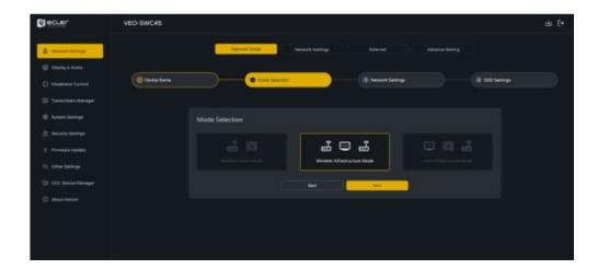
VEO-SWC45 can simultaneously connect to a wired and a wireless network. The segmented dual network of VEO-SWC45 provides two separated routing ways to connect to the base unit at the same time. This is very useful for organizations, which have a wireless "Guest" network for external visitors and a wired "Staff" network for their employees. Guest-users are not able to access any resource on the internal network of the company. Guest and Staff have internet access.
