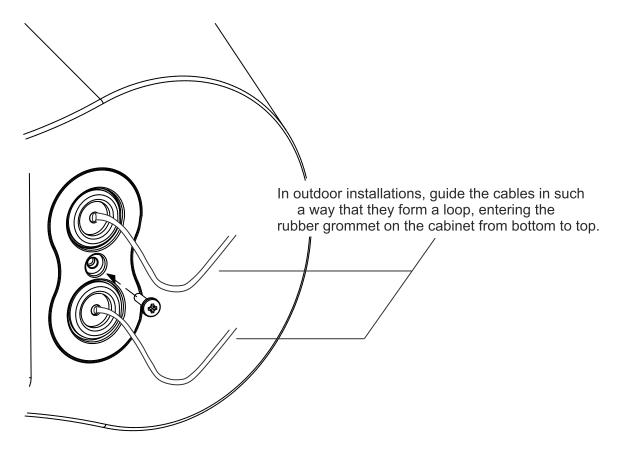
In outdoor installations, use a round tool to drill the grommets. Avoid making straight cuts. Additionally, ensure the use of round profile cables instead of parallel cables.
