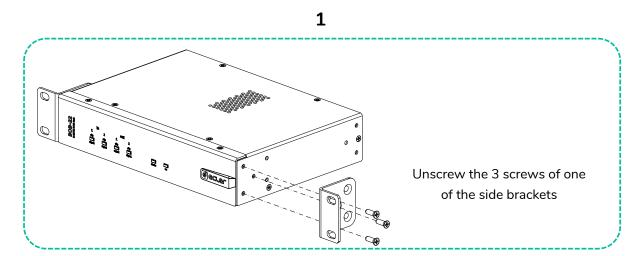
To attach the supplied front half-rack adapter, use the same 3 screws previously removed
