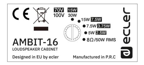
AMBIT-16, has 4 power handling levels for the 70/100V lines. Depending on the intended use, the speaker output can be attenuated more or less. In the zones where sound intensity should be low, place the switch in the 2.5W or 3.75W position. If sound intensity should be high, place the switch at 7.5W/15W.
