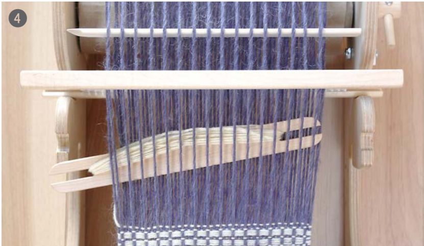
To use the pick-up stick to create a shed, put the heddle in neutral and flip the pick-up stick on its edge so it lifts up only the picked up ends.
