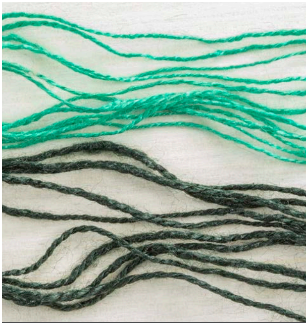
Devin used two spinning techniques to create samples. The light-green sample was spun with a semi-supported long draw from the fold, and the dark-green sample was spun with a short draw from the tips of the combed top.
