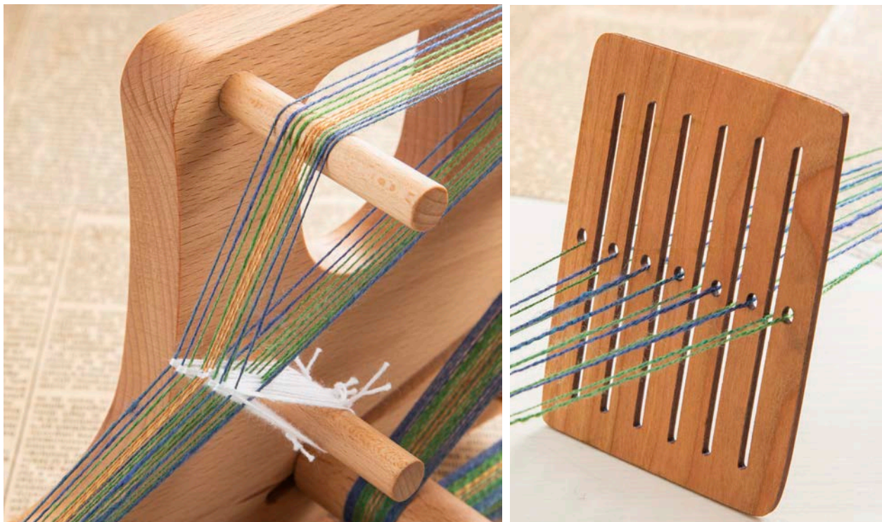
Inkle looms ( left ) typically function by anchoring every other thread with a heddle, keeping the warp closely spaced. Rigid heddles used with backstrap weaving ( right ) space the warp threads through a series of slots and holes. Shown here: Treenway Silks dyed tussah (see page 29), Ashford Inkleette, and Dancing Goats cherry rigid heddle.
