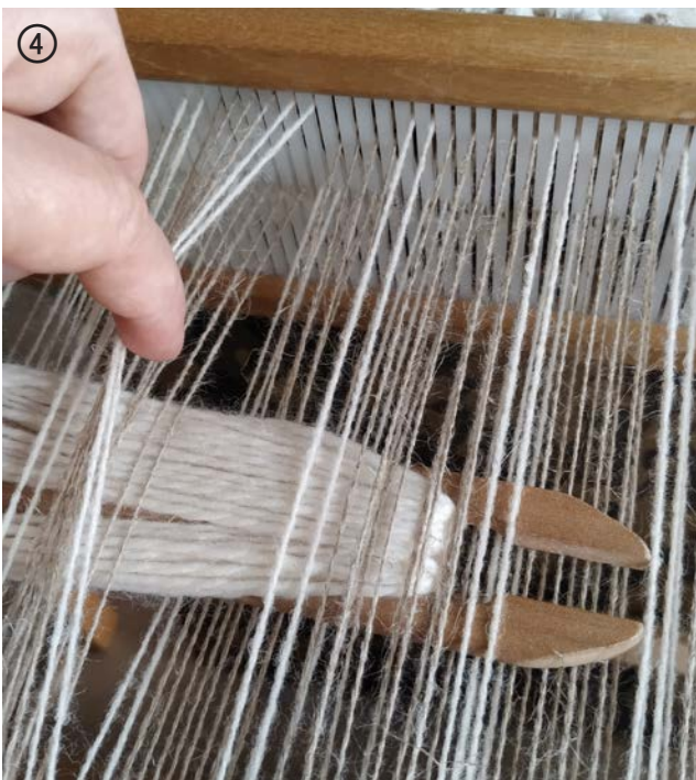
Photo 4: When weaving with the wool weft, Petra alternated picking up and pushing down the blocks of linen warp ends. Picking up the warp ends creates linen warp floats on the front and wool weft floats on the back, while pushing them down creates wool weft floats on the front and linen warp floats on the back.
