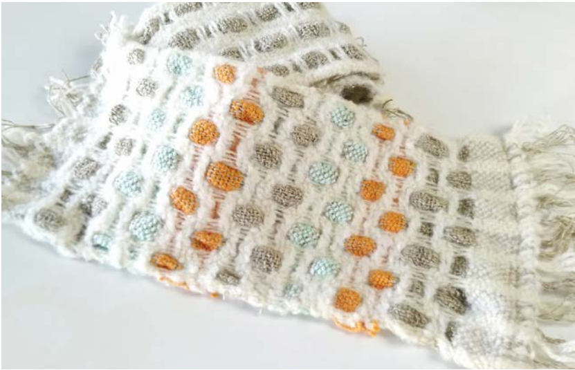
These two deflected-doubleweave swatches showcase the texture and weight of the finished samples. Using different non-shrinking wefts, adjusting the block sizes, and fulling the yarn more or less will change the weight and drape of the final fabric.
