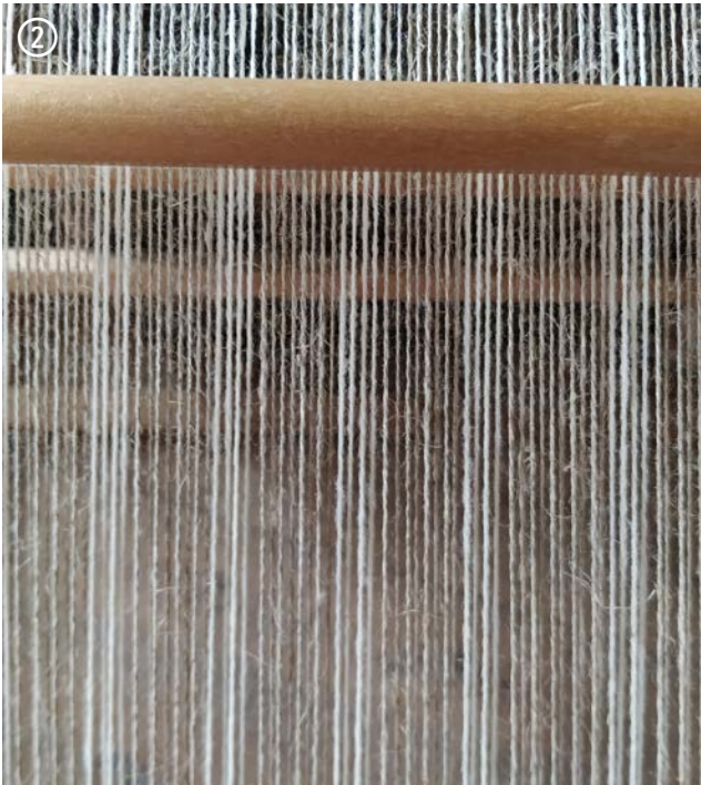
Photo 2: For her warp, Petra alternated 4 ends of white wool with 8 ends of natural-colored linen to create shrinking and nonshrinking blocks. Because the two warp yarns have different rates of elasticity, the tension of the warp will be uneven; however, the tension differences will not matter once the piece is wet-finished and differential shrinkage occurs.
