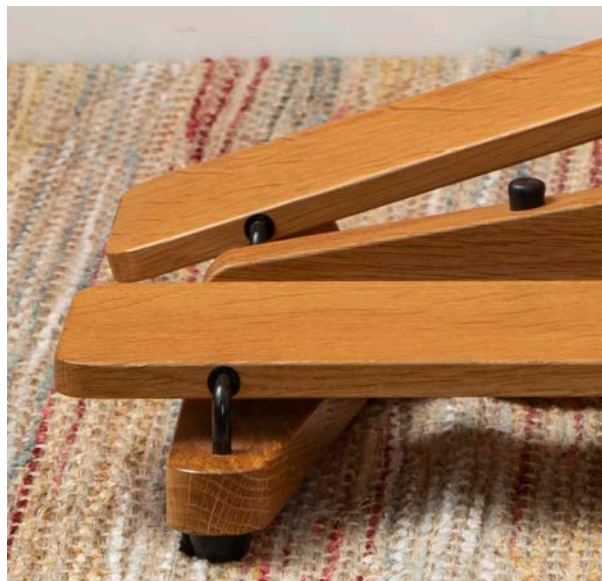
This treadle axis location allows for dorsiflexion, which means that the heel can push down and contribute to the treading action. This can be helpful for spinners with certain sensitivities in the feet and legs.
