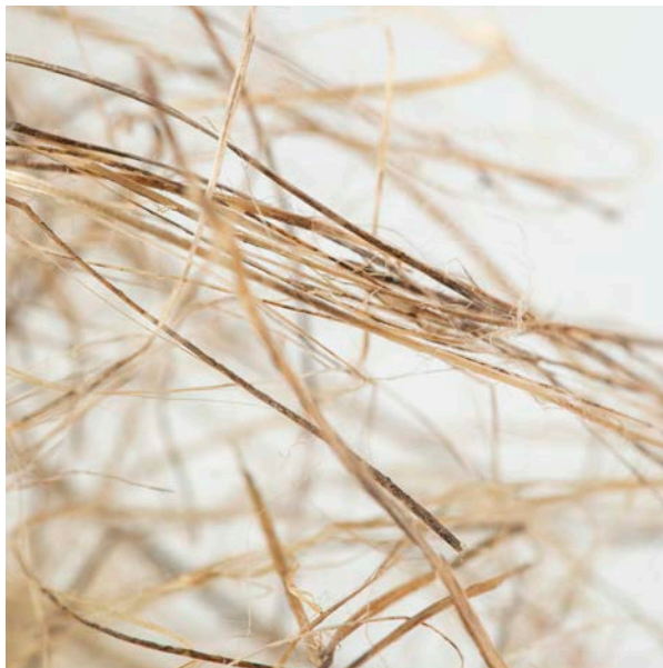
Retted hemp before cottonization. Pectins and lignins hold many short fibers together in long strands of bast.
