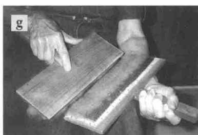
f & g. After transferring (step 3), Gladys continues to card. But following each transfer, she allows a little bit less of the fiber from the right card back onto the left card.
