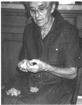
Hand-ginning cotton consists of pulling the fibers away from each seed.
