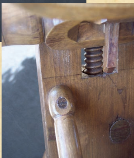
The wooden tension screw in the table is hand-turned. The metal screw was added during restoration.
