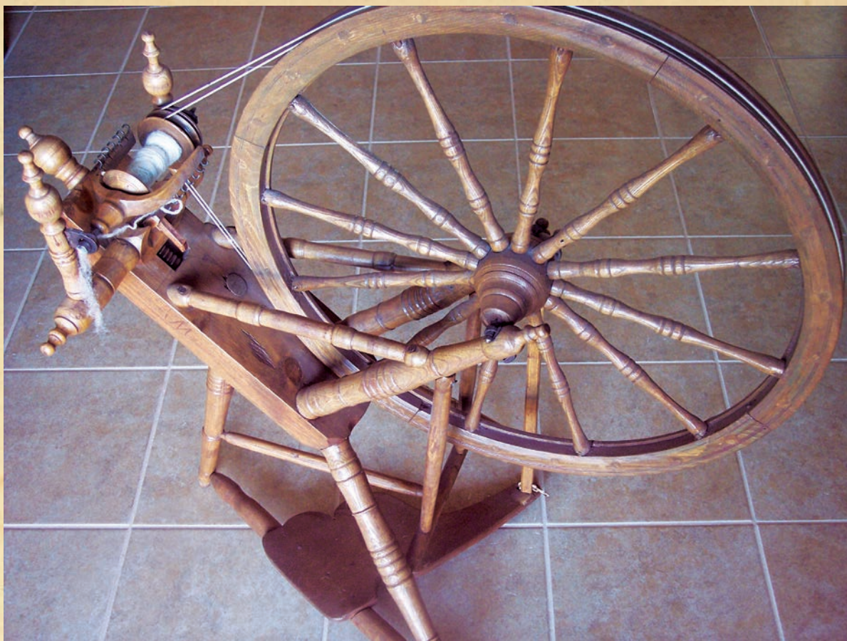
Lars Moen's handmade spinning wheel was held together using glue and pegs.
