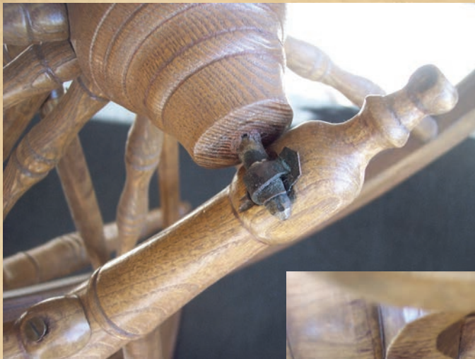
A hand-shaped metal bearing holds the axle of the wheel's hub.
