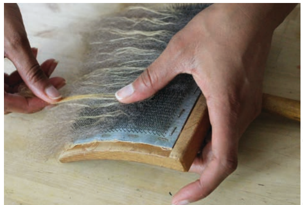
Heavenly applying a thin layer of eri silk on top of wool before handcarding.
