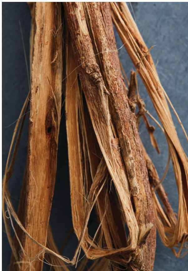
After retting for only nine days, the fibers are just beginning to be released from surrounding plant matter.
