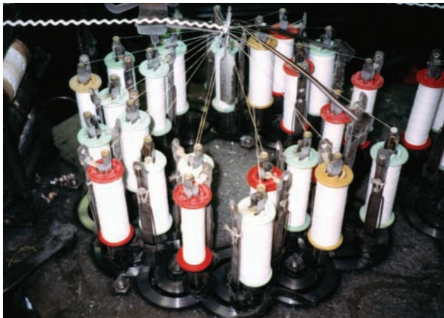
A German-designed braid machine weaving rickrack at the Trimtex Company. Note that the threads converge at a central point at the top, where the weaving occurs. Photograph courtesy of Trimtex Company Inc., Ridgefield, New Jersey.
