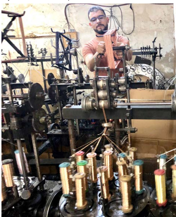
Cleverly devised braiding machines make sfifa embellishment affordable for the less affluent.
