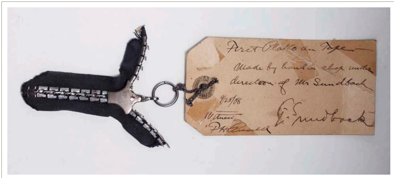
"First Plako on tape—Made by hand in shop under direction of Mr. Sundback. 9/25/08" Object from the personal records of Gideon Sundback. Courtesy of Special Collections, Pelletier Library, Allegheny College
