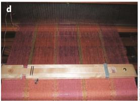
To adjust temple width: Put the temple on its side. Place the base of the teeth at the edge of the warp in the reed on both sides of the warp (a). Place the pivot pin in the hole that secures this width. Insert the teeth into the left selvedge, one to two warp threads inside the edge thread (b): do the same thing on the opposite selvedge. Gently push down on the center bar (c). Move the metal slider to secure the center bar (d). Very important: Advance the temple every 1½".
