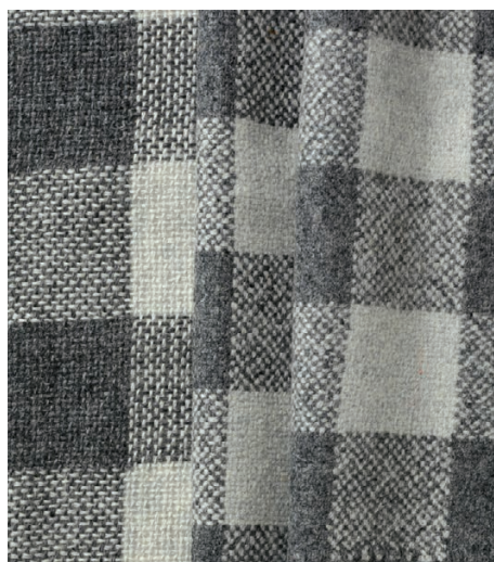
c. Plain weave at 10 epi (left to right): unfinished, fullled 25 min, fullled 70 min.
