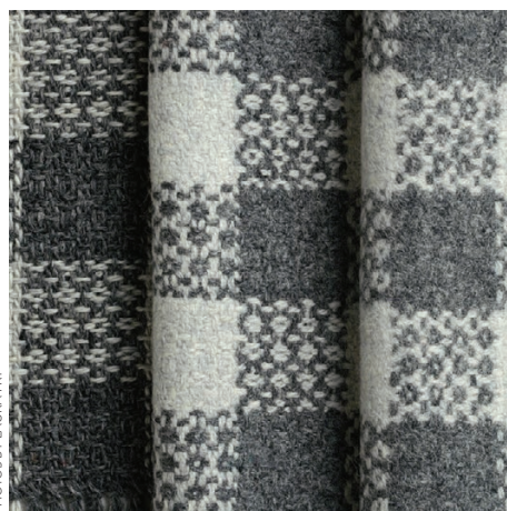
e. Point twill at 16 epi: unfinished, fullled 25 min, fullled 70 min.
