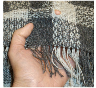
b. Before wet finishing, the cloth is loose enough that the threads can be separated. Fulling causes the fibers to cling to each other for stability.
