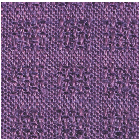
Sample e (left): unfinished 20/2 spun silk woven in huck lace stripes at 24 epi and ppi.
