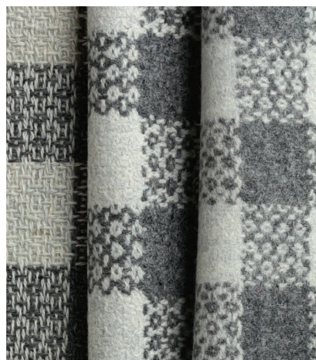
d. Point twill at 12 epi: unfinished, fullled 25 min, fullled 70 min.
