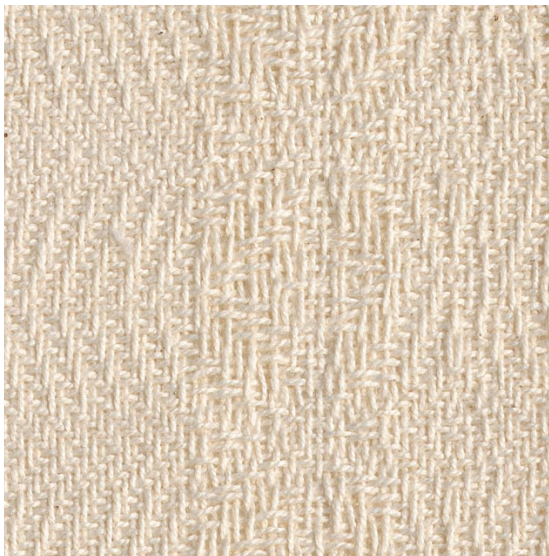
Sample a (left): unfinished 8/2 unmercerized cotton woven in an advancing twill at 24 epi and ppi. Sample b (right): the same cloth, wet finished.
