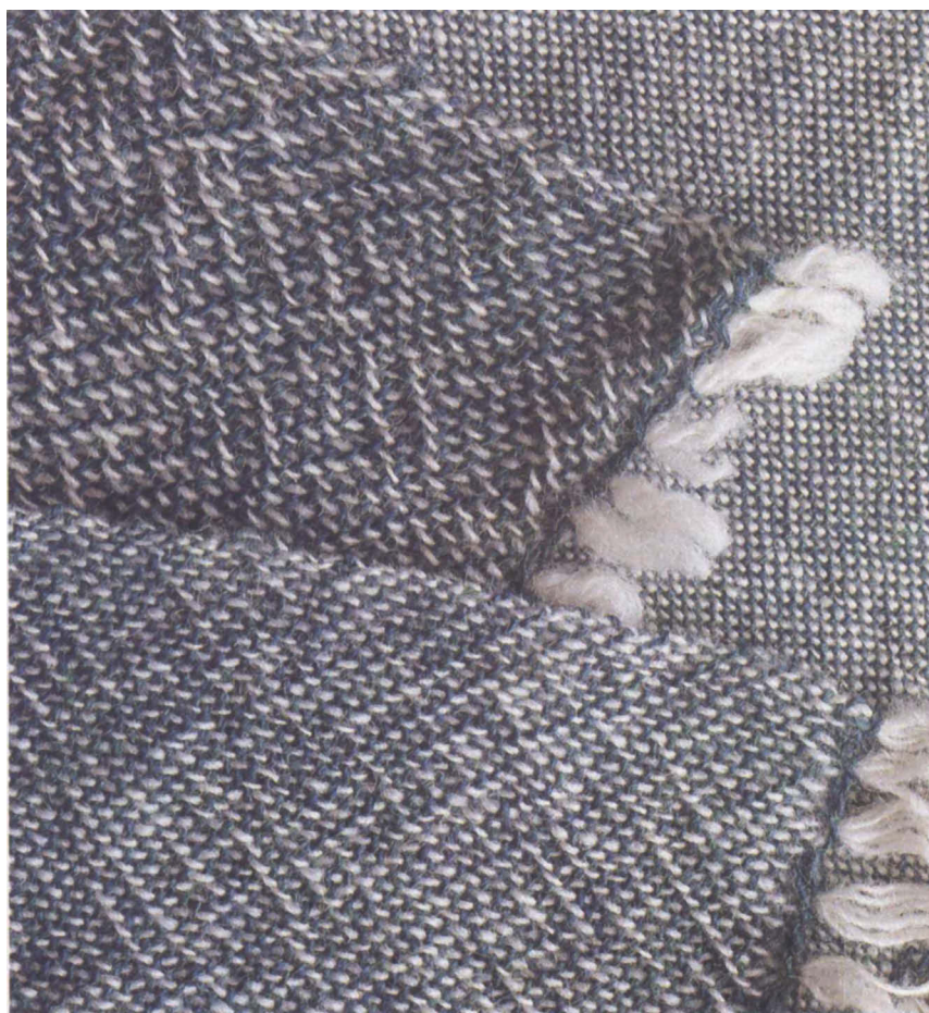
Three samples of plain weave fabrics. From the top down: 18 e.p.i./p.p.i., washed but not pressed; there is no observable tracking. 10 e.p.i./p.p.i., washed but not pressed; there is extreme tracking. 12 e.p.i./p.p.i., washed but not pressed; tracking is very pronounced.
