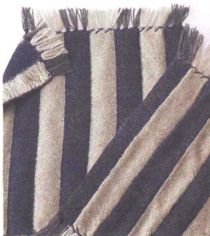
Top swatch: 6-shaft, true Bedford cord. No slippage occurs at edges of cords. Bottom swatch: 4-shaft Bedford cord with no cutting ends. Note slippage at edges of cords.
