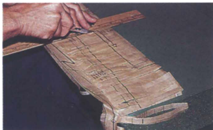
Photo 1. The 1" selvedge is folded over the edge of the cutting board and then cut through the fold nearest the selvedge through the fold at the top.
