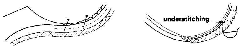
Illustration 7. Stitch bias facing to main fabric edge, right sides together. Clip any curves (left). Turn facing and main fabric to inside, stitch seam allowance to facing (understitching). Hand stitch facing (right).
