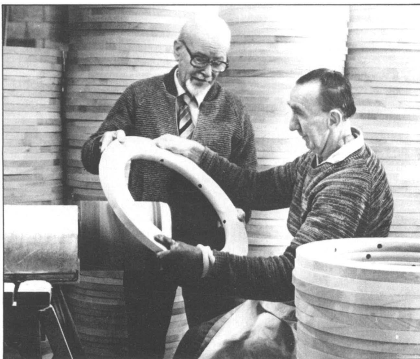
Walter Ashford (left), designer of the original Ashford Spinning Wheel, still keeps an eye on every stage of the manufacture. Here, surrounded by stacks of wheel rims, he checks out the sanding operation.
