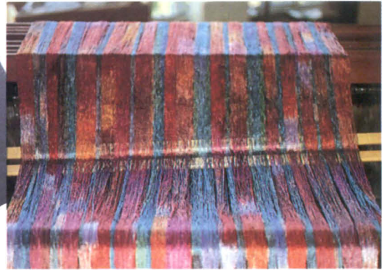
Beaming the painted warp for the scarf shown here. Michele Wipplinger painted the warp for this scarf using the technique described below. Her yarn is 8/2 "carpet" silk from Treenway set at 40 e.p.i.
