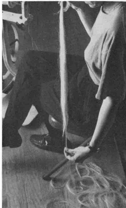
Making a flax roving by attenuating fibers from a "finger" of flax.
