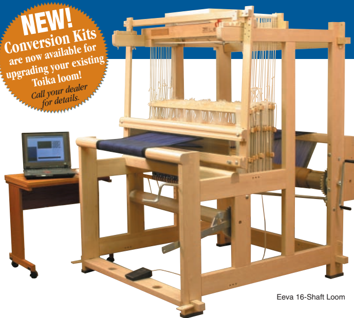
Toika Computer-Controlled Looms are powered by WeavePoint 6.0 software, which runs on any computer equipped with Windows 95, 98, 2000, or XP.
