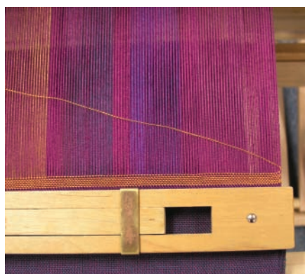
a. Set the temple at the width of the warp in the reed. Insert weft threads at an angle.
