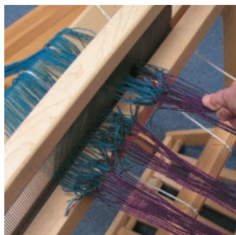
f. Shake the knots through the reed
