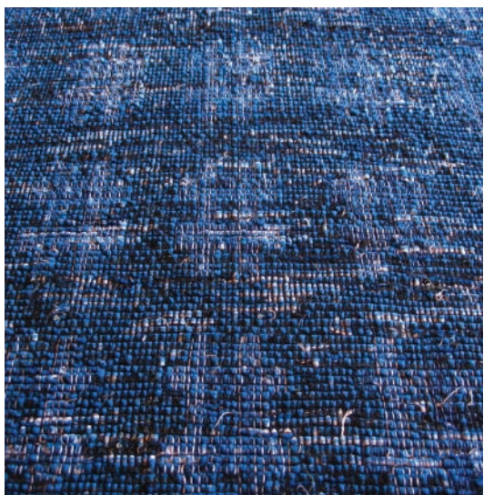
b. The 6-shaft draft woven with another kimono fabric weft
