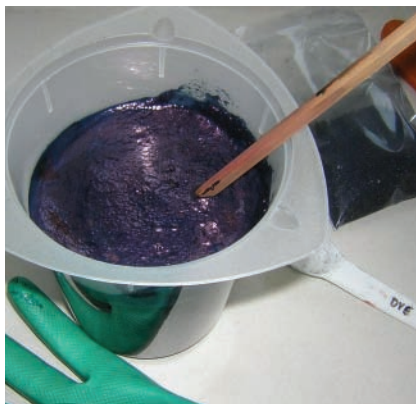
c. One quart of warm water is mixed with powdered dye (wear dust mask and gloves).
