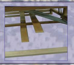
Exceptionally easy treadling eliminates the need for a complex and costly power assist mechanism and allowing the weaver to control the weaving speed. The distance between the top and bottom treadle is less the 8".
