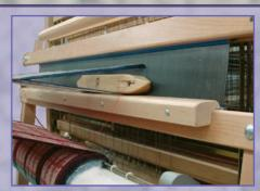
Our true countermarch system gives an equal tension on the top and bottom warp threads providing a large shed with lower stress on the warp.
