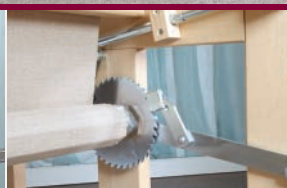
Linen aprons on the cloth and warp beams
