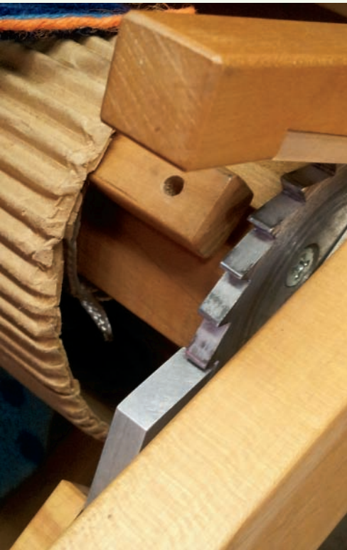
A ratchet-and-pawl braking system.
