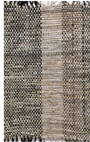
LEFT: paper linen and silk noil in plain weave, unwashed; RIGHT: paper linen and silk noil in plain weave, wet-finished and ironed.
