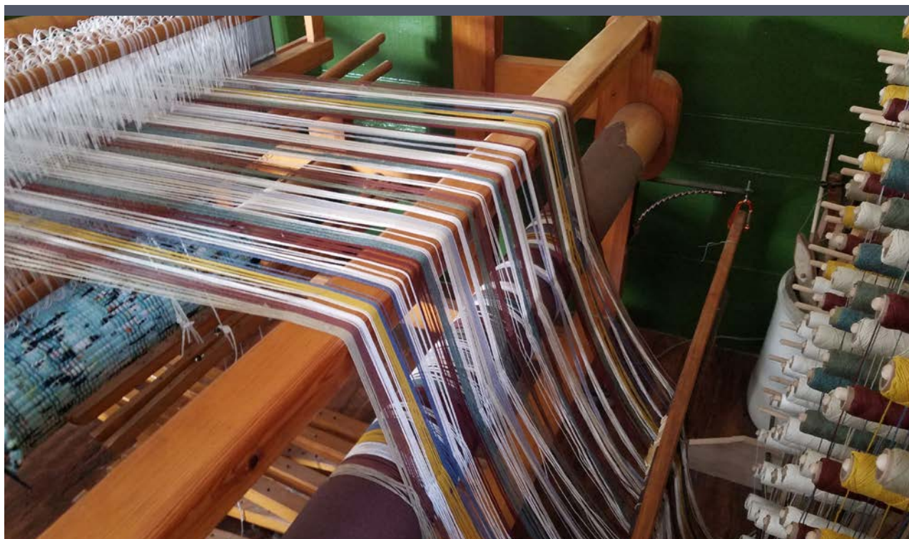
As Laura advances the warp, more yarn comes off the spools behind the loom, through a reed, around a beam wrapped in fine-grit sandpaper, through heddles, and through the front reed where it’s perfectly tensioned. This setup allows Laura to continuously weave about 800 yards before needing to rewarp.
