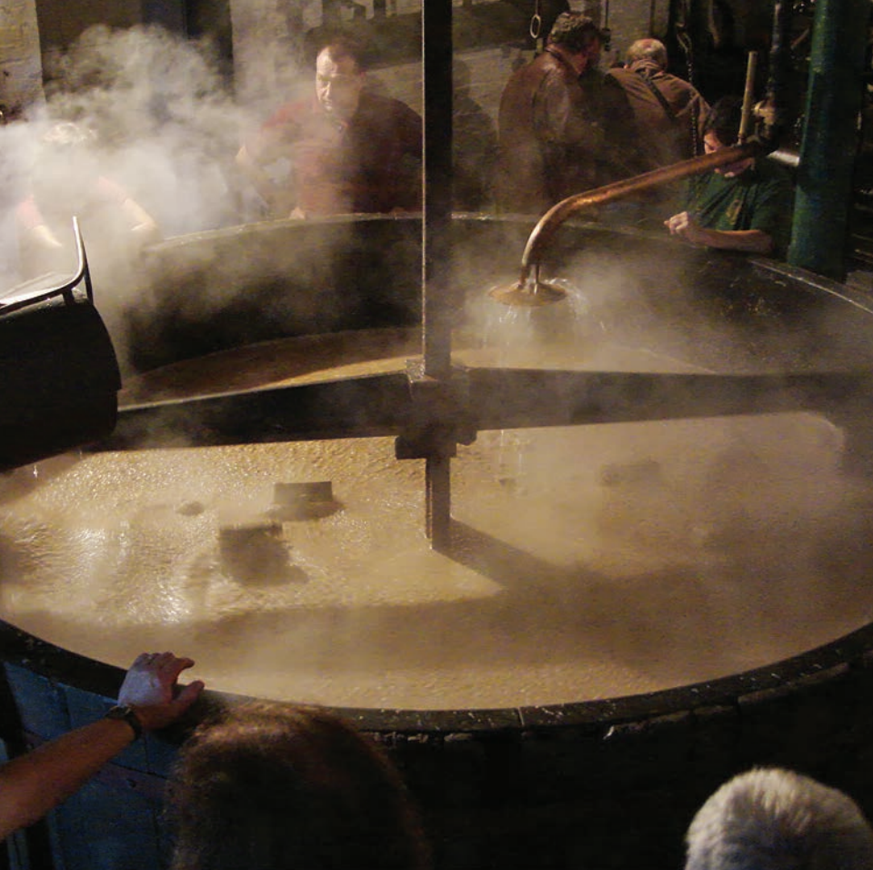
Steam still powers the mash tun at the Brasserie à Vapeur in Pipaix, Hainaut.
