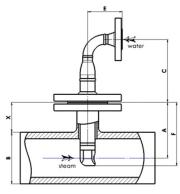
The variable dimension is X, in order to have the Sprayhead in the center of the pipe
